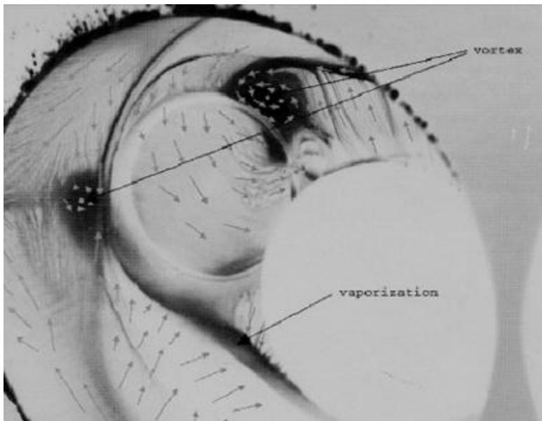
Image of vortices within a combustion chamber
