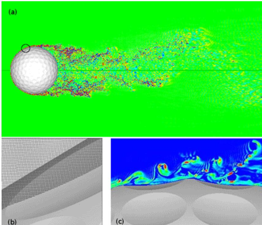
Above is the results of a "direct numerical simulation of the flow around a dimpled sphere at  $Re=110000$ . Figure (a) Side view of the wake visualized by spanwise vorticity isolines.; Figure (b) Detail of the mesh in a dimple; Figure (c) Visualization of the shear layers in a single dimple.<sup>3</sup>
