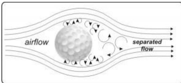
Illustration of the micro turbulence boundary layer created by dimples on a golf ball
